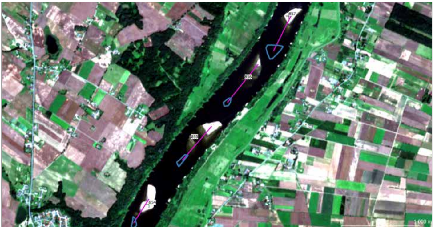
Fig. 3a. The shift of the sandbars on the lower Vistula channel between 854-857 km in the period from September 4, 2016 to July 30, 2017, measured on satellite Sentinel-2 images (source: A. Magnuszewski)
