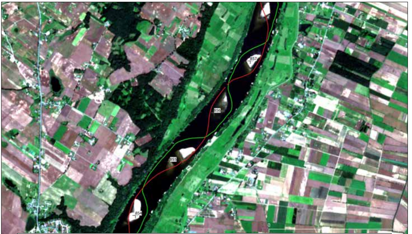
Fig. 4a. Lines of thalweg on the lower Vistula River between 854-857 km (red line 6 September 2016 and green line 14 July 2017) (source: A. Magnuszewski)
